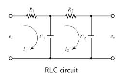
$$\frac{1}{C_1 s} [I_1(s) - I_2(s)] + R_1 I_1(s) = E_i(s)$$
