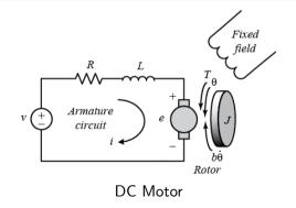
• For the armature electrical circuit KVL:
